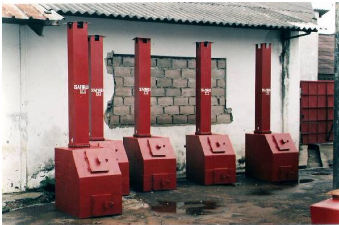
Picture 7. Metallic Incinerators
